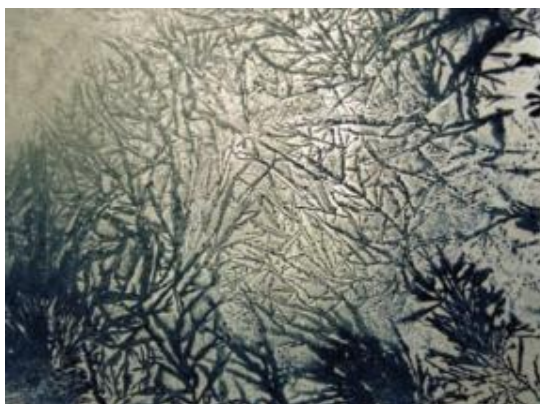
Figure 12: These are crystals formed after drying an aqueous solution of \text{CuCl}_2 through which a direct current of 10 mA was passed for 10 minutes [56]; compare with Figure 6, right.
