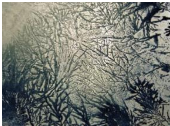
Figure 2: These are crystals formed after drying an aqueous solution of \text{CuCl}_2 through which a direct current of 10 mA was passed for 10 minutes [15]; compare with Figure 1, right.
