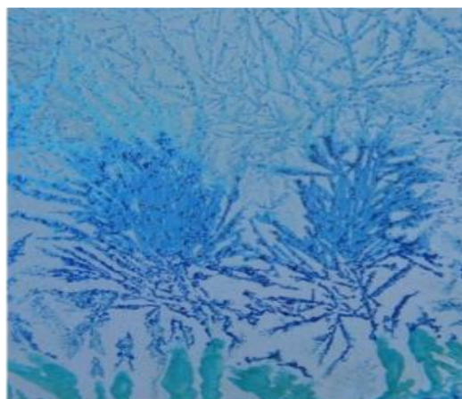
Figure 3: These are crystals formed after drying an aqueous solution of \text{CuCl}_2 , which was previously subjected to the action of EMF, pulsing with a frequency of 10 Hz for 10 minutes; for contrast, the crystals formed were treated with ammonia vapours [15]; compare with Figure 1, right.
