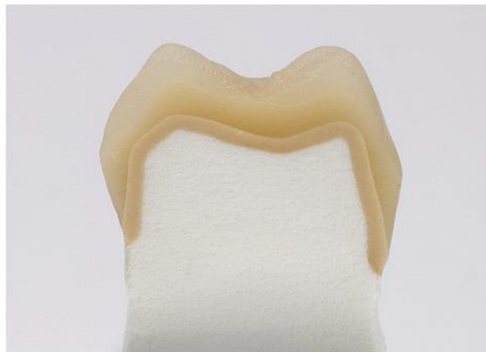
Figure 1: CICERO®: Digitally veneered alumina coping [11].
