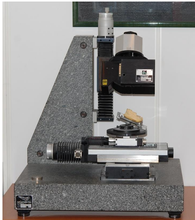
Figure 2: CICERO®: First laser-line laboratory scanner [12].
