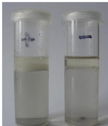
Figure 5: Suspensions formed by intensive mixing of oils with positively charged water do not stratify for hours and, accordingly, retain their milky white or yellowish colour (left), unlike suspensions formed by intensive mixing of the same oils with negatively charged water, which stratify within minutes (right) [4].
