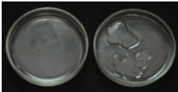
Figure 1: Left: The low surface tension of negatively charged water does not limit its spreading and allows it to completely cover the bottom of the Petri dish. Right: The high surface tension of positively charged water causes it to be compressed and therefore prevents it from spreading [1, 2].
