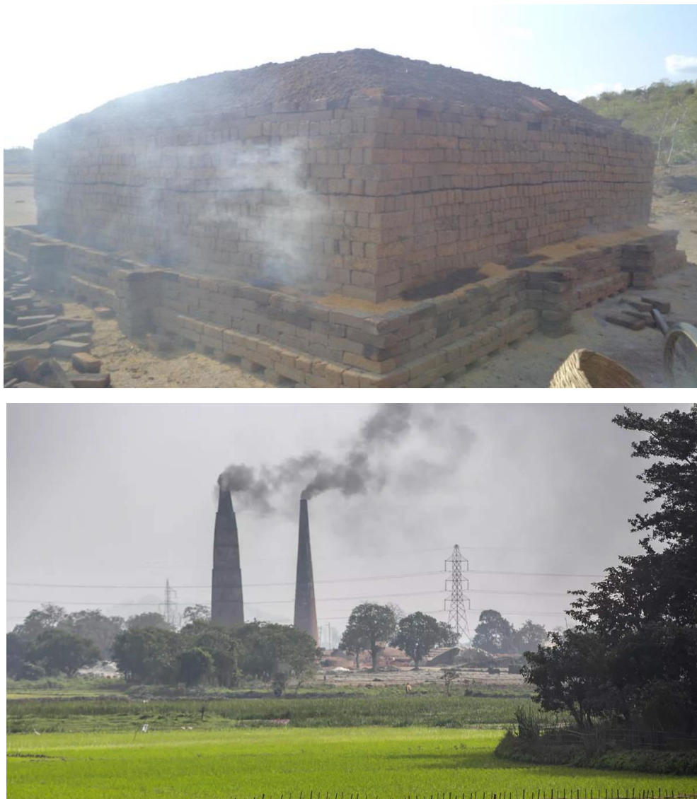
Figure 1. Old or traditional (a) and modern or fixed chimney bull's trench (b) coal-fired brick kilns in India.
