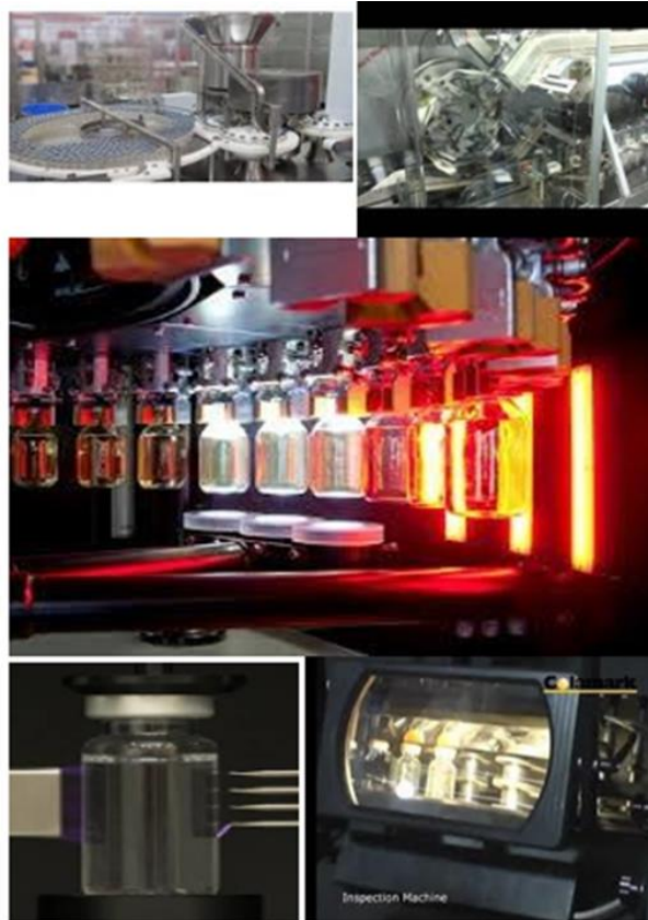
Particle inspection in liquid product
