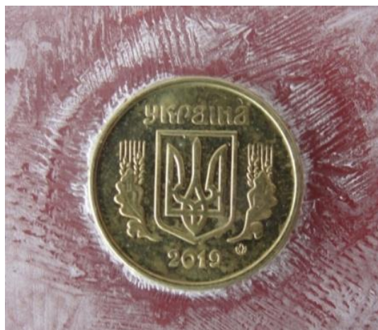
Figure 5. This is a "copper" coin surrounded by a dried MgSO 4 solution prepared in uncharged water; in this case, needle-shaped crystals also form around the coin.
