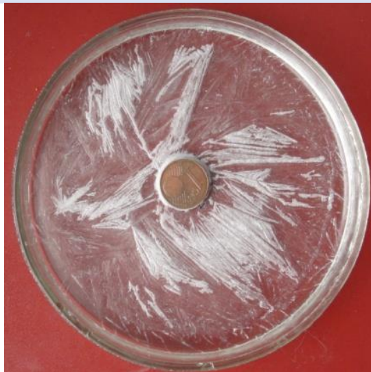
Figure 4. This is a "copper" coin surrounded by a dried K 2 CO 3 solution prepared in uncharged water; in this case, distinct needle-shaped crystals form around the coin [39].
