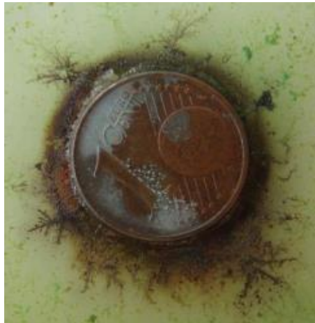
Figure 6. This is a "copper" coin surrounded by a dried CuCl_2 solution prepared in uncharged water; in this case, distinct plant-type crystals are formed [39].
