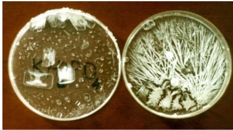
Figure 1. It is the crystals that formed after the drying of solutions of \text{KH}_2\text{PO}_4 prepared on the water with potentials of +250 mV (left) and -250 mV (right) [29].
