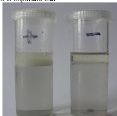
Figure 5. Suspensions formed by intensive mixing of liquid oils with positively charged water do not delaminate for several hours, retaining a milky white or yellowish colour (left); suspensions formed by intensive mixing of the same oils with negatively charged water separate within minutes (right) [3-5].
