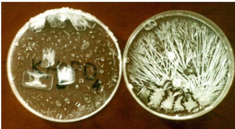
Figure 1: It is the crystals that formed after the drying of solutions of \text{KH}_2\text{PO}_4 prepared on the water with potentials of +250 mV (left) and -250 mV (right) [1, 2].
