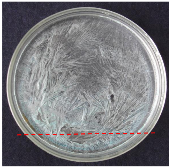
Figure 17: These are needle-shaped crystals formed after the drying of an aqueous solution of \text{CuSO}_4 located under a wire with a pulsed electric current with a frequency of 2 Hz (dashed red line); it is worth noting that these needles are directed away from the wire.
