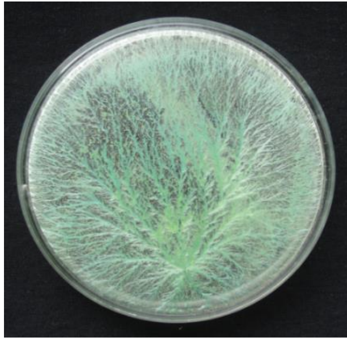
Figure 11: These are filaments formed in a glass Petri dish after drying a \text{CuCl}_2 solution prepared in negatively charged water [4].
