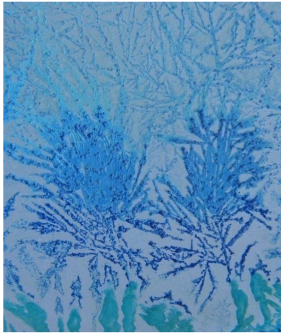
Figure 7: The crystals formed after drying an aqueous solution of \text{CuCl}_2 , which was previously subjected to the action of EMF, pulsing with a frequency of 10 Hz for 10 minutes.
