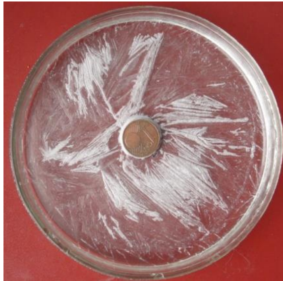
Figure 15: This is a "copper" coin surrounded by a dried aqueous solution of K_2CO_3 prepared in negatively charged water.
