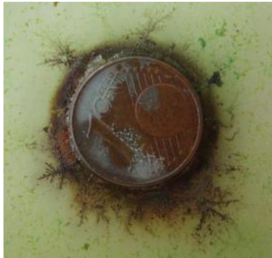
Figure 16: This is a corroded "copper" coin surrounded by a dried aqueous solution of CuCl_2 prepared in negatively charged water.
