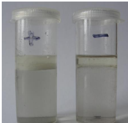
Figure 7: Suspensions formed by intensive mixing of liquid oils with positively charged water do not delaminate for several hours, retaining a milky white or yellowish colour (left); suspensions formed by intensive mixing of the same oils with negatively charged water separate within minutes (right) [13-15].
