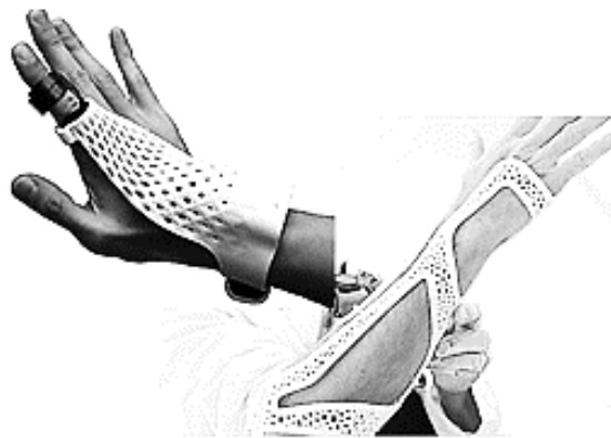
Figure 6: Sample schematics of auxetic SMM actuator for arm muscular skeletal motion
