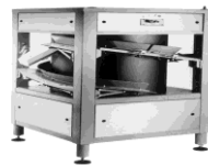
Figure 27: Typical conical rounder
