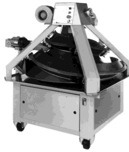
Figure 26: Typical conical rounder, note this model has operator adjustable tracks
