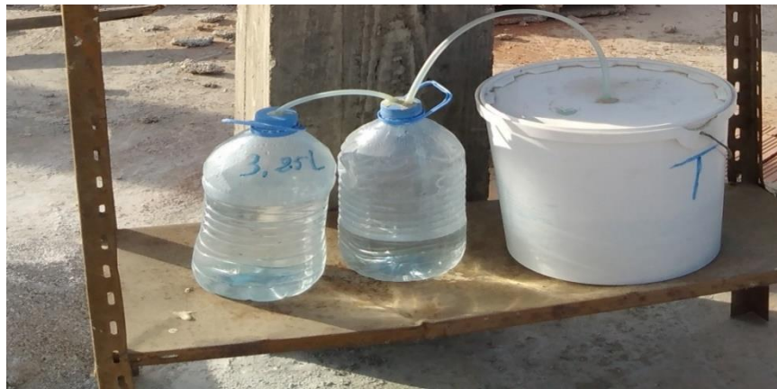
Figure 05: The digester used.
