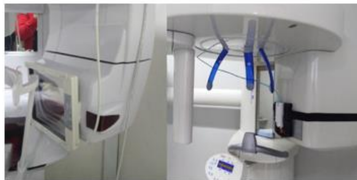
Figure 2: Experimental settings for the product medidas kerma aire-area, PKA, (izquierda) and exposure parameters in panoramic radiography equipment (derecha).
