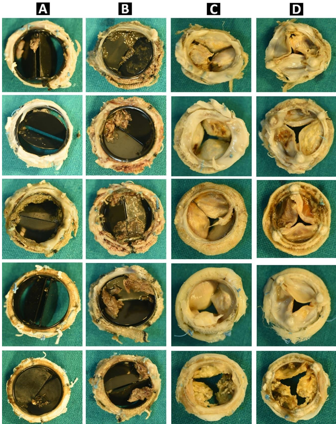
Figures 7A-7D: Photographs of explanted St. Jude mechanical valve with thrombotic occlusion of leaflets (A, B) and PERIMOUNT bioprostheses (C, D) showing structural valve deterioration (Cuspal perforation, tear, thickening, calcification, stiffness, wear and abrasions, creep, and stress fracture).
