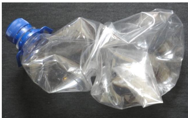
Figure 1. So it looks like a closed PET bottle with hydrogen gas a two weeks after filling it. The changes that have taken place with the bottle show that hydrogen gas freely penetrates through the plastic [3].
