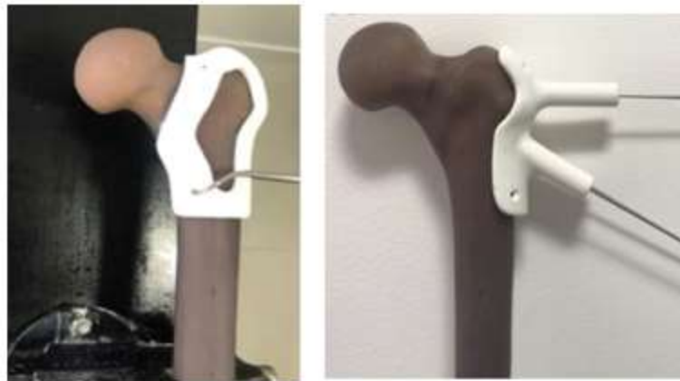
Figure 1: Osteotomy 3D printed guide (left) and a 3D printed guide to position the cannulated screws.
