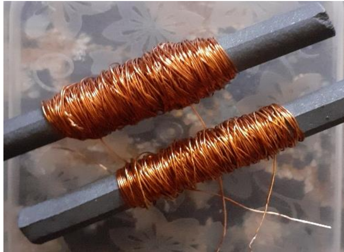
Figure 16: Primary and secondary windings. The number of turns of the primary winding is 180 turns and the secondary winding is 340 turns.
