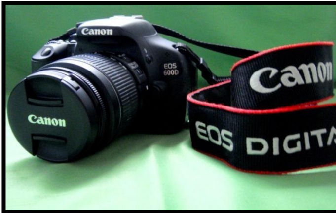
Figure 2: Canon EOS 600 DSLR Camera, 18Megapixels, image sensor 22.3X14.9mm, 18-55mm macro lens with image stabilize.
