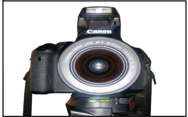
Figure 5: Camera mounted on the tripod. Fluid level device attached to the head of the tripod
