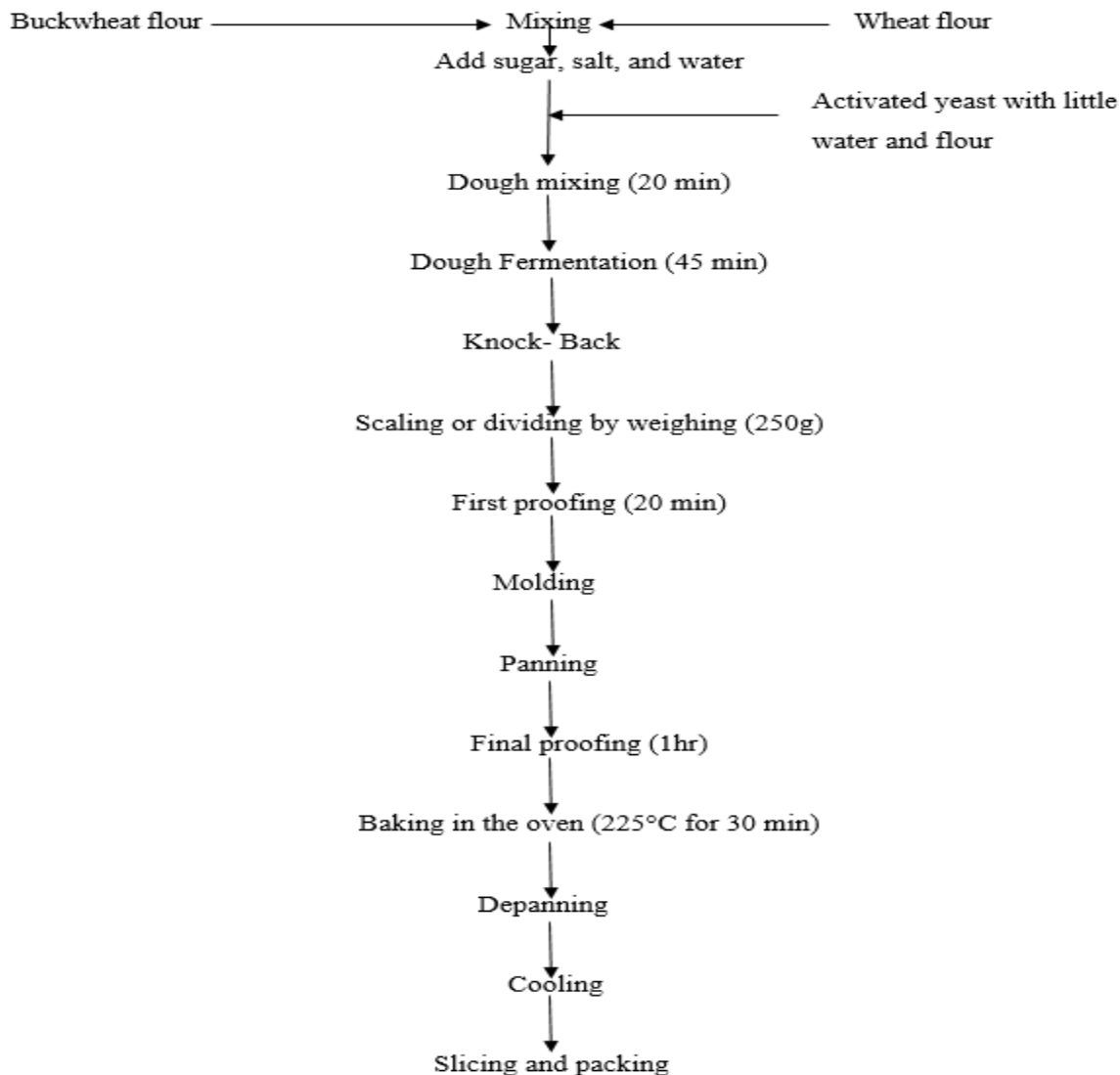
Figure 1. Flowchart of bread making process
