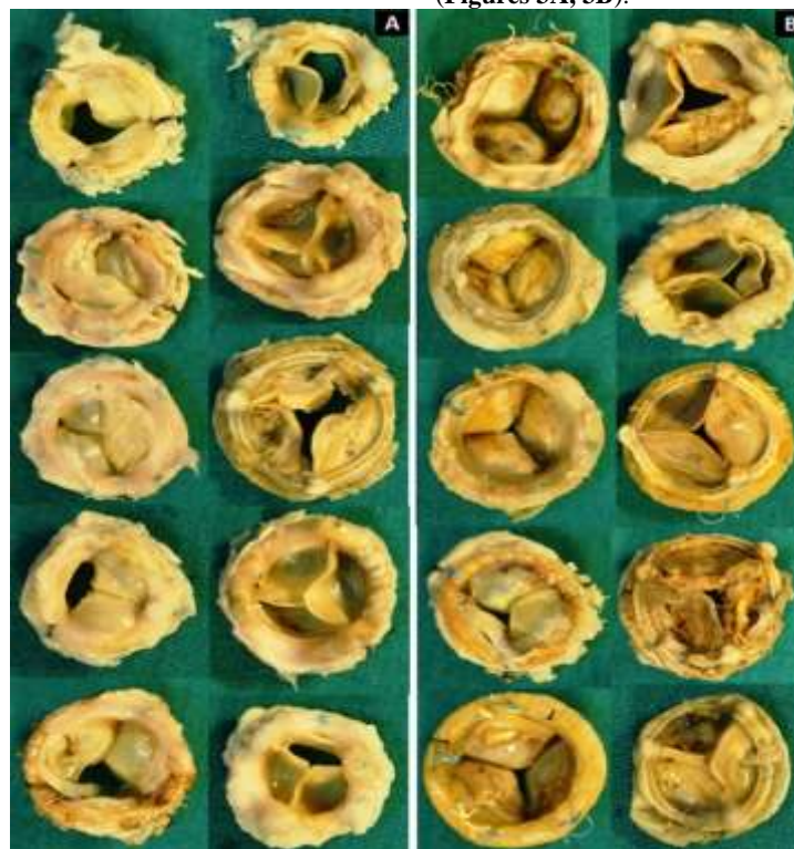
Figure 3A, 3B: Photographs of explanted Epic (Figure 3A) and PERIMOUNT (Figure 3B) mitral bioprostheses showing different types of structural valve deterioration (Cuspal perforation, tear, thickening, calcification, stiffness, wear and abrasions, creep, and stress fracture) [A-Atrial surface; B-Ventricular surface]
