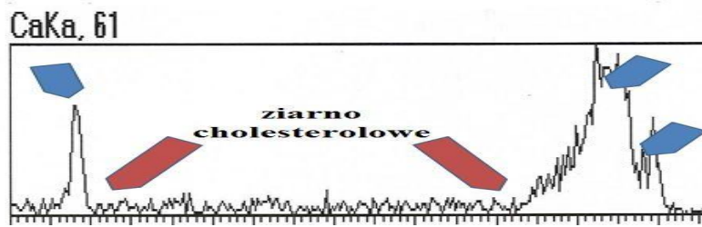
Figure 1: Sample E. Chemical analysis graph for grain mineralization. Elevated levels of calcium (blue arrows) at the edge of cholesterol grain (red arrows). SEM, linear measurement. Scale – micrometers.
