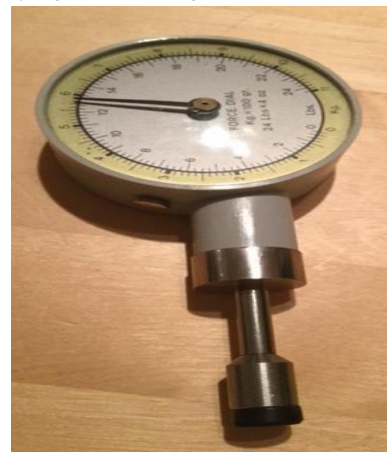
Figure 1. A Fischer Probe is a pressure algometer, increasing pressure on the skin at a constant rate until the pain threshold is reached and the current pressure is measured.
